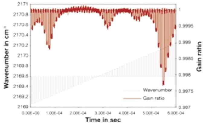
*Circuit simulation results: the wavelength is scanned in steps (blue square-wave) across a CO absorption line (2169.2 cm<sup>-1</sup>) and a nearby CO<sub>2</sub> line (2170.2 cm<sup>-1</sup>). The red signal is the gain ratio, showing the detection of both species during a 0.6msec scan.*
